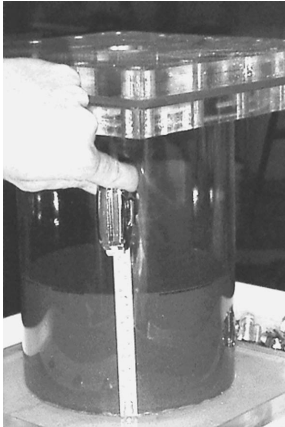
Fig. 8. Acrylic modeling box with sediment and cap.
